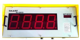
The instrument is single Microcontroller based, SWITCH MODE POWER SUPPLY UNIT (SMPS), REMOTE KEYPAD / software for programming & counter setting & resetting, seven segment display unit for displaying RUNNING COUNT/PRESET COUNT.
